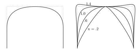
A straight line is drawn along the first half of the first segment and the last half of the last segment. The curve is tangent to the centres of the segments. The dpic result of including an expression after spline, as in
